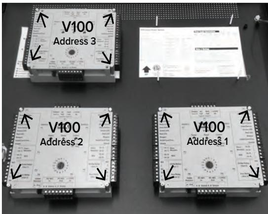
8. Using a small slotted screwdriver gently turn the V100 addresses as follows:
